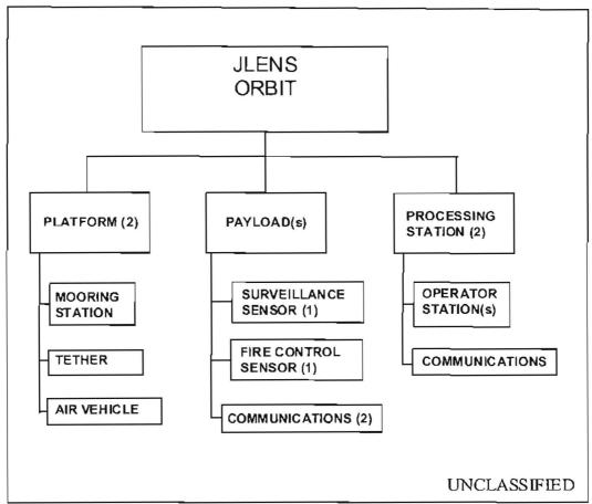
Figure 1.3-1. (U) JLENS System Specification Tree
